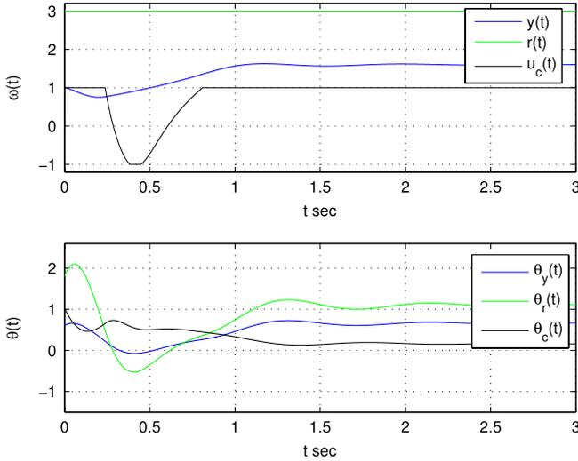
**Fig. 4.** Simulation of the adaptive control system for the plant (17) and the controller (6), for the case when  $r(t) = 3$ . The upper and lower graphs show the time history of the regressor  $\omega(t)$  and the adaptive gain  $\theta(t)$  vectors, respectively.
