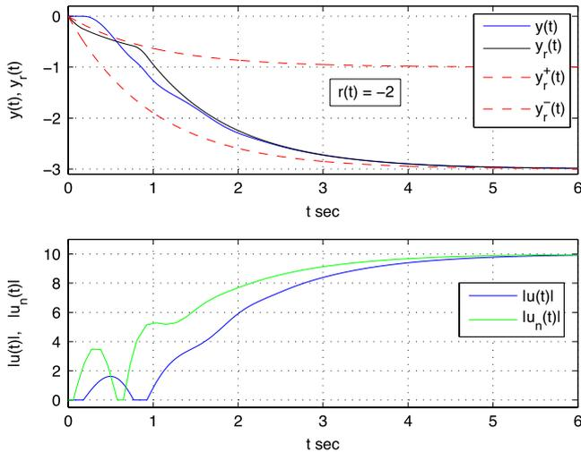
**Fig. 5.** Simulation of the adaptive control system for plant (29) and controller (23). The upper graphs show how the adaptive controller finds a reference trajectory within the admissible range  $y_r^- \leq y_r(t) \leq y_r^+$ . The lower graphs show the time history of the absolute value of the control signals  $|u(t)|$  for the cases of adaptive control with (blue lines) and without (green lines) optimization, respectively.
