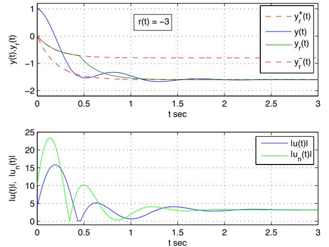
**Fig. 3.** Simulation of the adaptive control system for plant (17) and controller (6). The upper graphs show how the adaptive controller finds a reference trajectory within the admissible range  $y_r^- \leq y_r(t) \leq y_r^+$ . The lower graphs show the time history of the absolute value of the control signals  $|u(t)|$  for the cases of adaptive control with (blue lines) and without (green lines) optimization, respectively.
