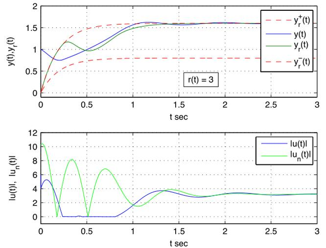
**Fig. 2.** Simulation of the adaptive control system for plant (17) and controller (6). The upper graphs show how the adaptive controller finds a reference trajectory within the admissible range  $y_r^- \leq y_r(t) \leq y_r^+$ . The lower graphs show the time history of the absolute value of the control signals  $|u(t)|$  for the cases of adaptive control with (blue lines) and without (green lines) optimization, respectively.
