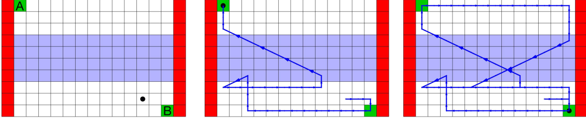
Fig. 3. Case Study 1: (Left): The Robot (shown in black) and its environment. (Middle): Snapshots of the executed Motion at time k = 33 , and (Right) k = 62 . The robot satisfies the specification.
